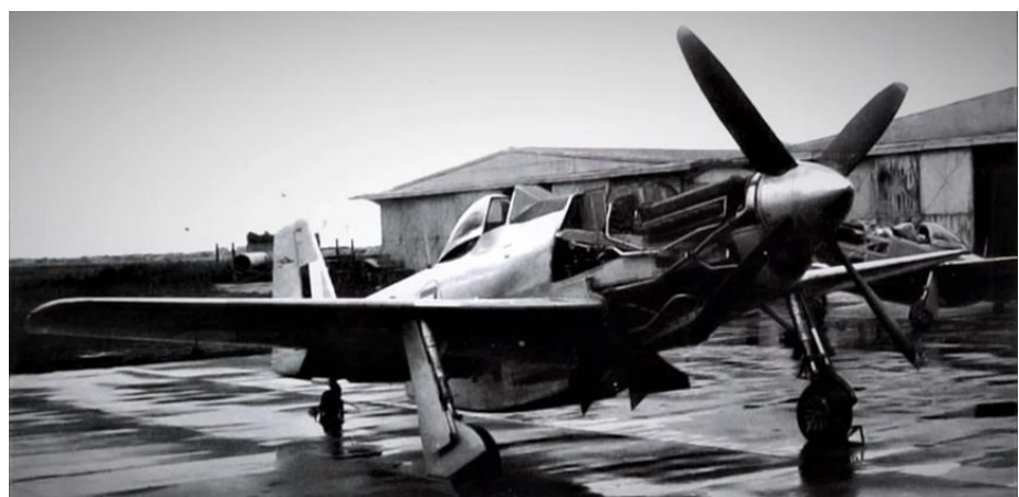
CA-15 with engine cowling removed, showing the Rolls-Royce Griffon engine.
