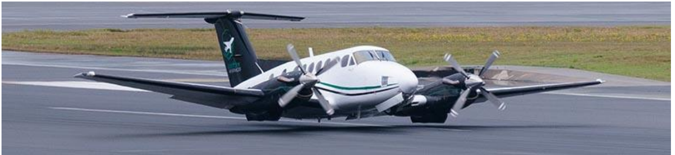
Beechcraft B200 Super King Air VH-XDV conducts an emergency, wheels up landing at Newcastle airport, NSW
