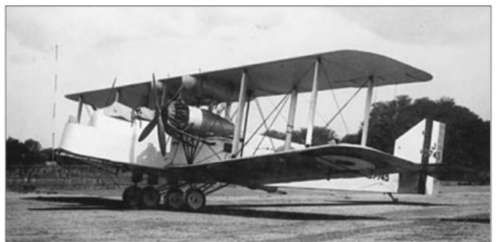
The Hinaidi which participated in the airlift was J7745, the original prototype Hinaidi 1, which had been converted from a Hyderabad. For service in tropical conditions, it had been given an overall aluminium dope finish.
