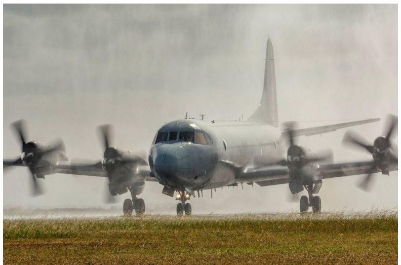
An AP-3C taxis through a 'bird bath' which is used to wash salt water off the aircraft after low level flights over water.
